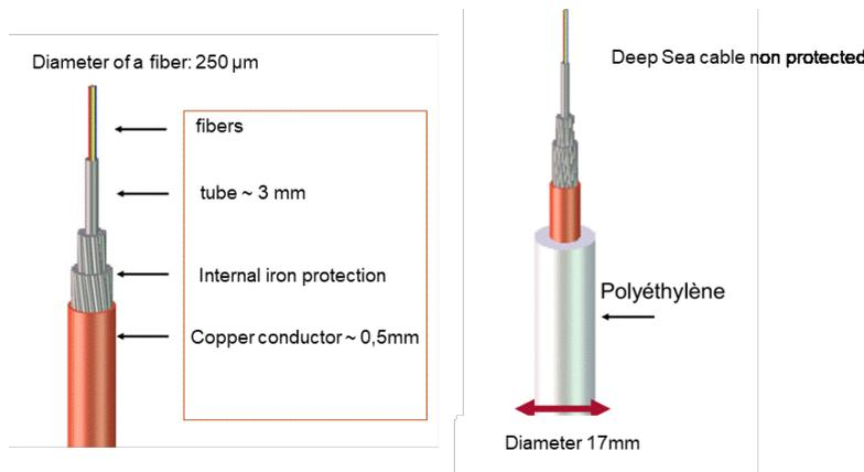
From right to left <sup>72</sup>, from no armour (for the deep sea) to double armoured (for shallow waters).
